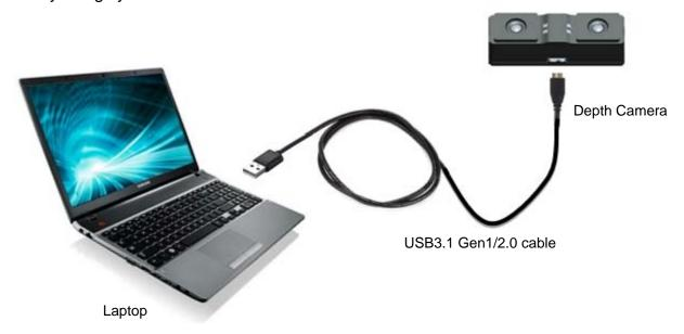
Figure 3-1. Depth Camera to PC Connection
